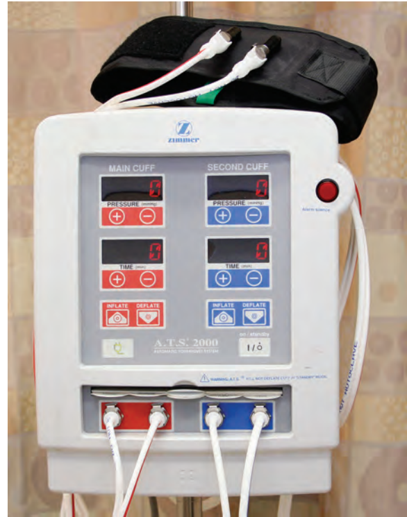
Figure 32.2 A digital-controlled double-cuff system by Zimmer (A.T.S. 2000, Zimmer Inc., Bloomfield, CN) allows safe intravenous regional anesthesia and the ability to lessen pain from the arterial tourniquet.
