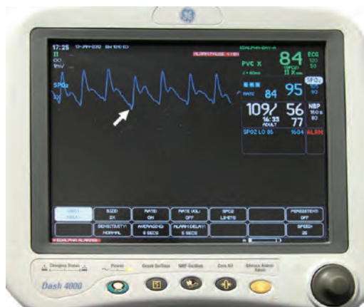
Figure 2.8 Patient monitor displaying a pulse plethysmograph ( arrow ). The patient's heart rate (84) and O 2 saturation (95) are also displayed ( blue numbers ).
