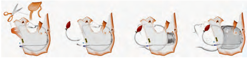
Figure 46.36 The Eject Helmet Removal System. This device uses a small air bladder that is neatly folded in an accordion fashion and placed underneath the helmet liner. A small tube runs under the padding and fastens to the bottom of the rim of the helmet to provide easy access. The device may be prefitted into the rider's helmet or inserted at the time of removal by using an insertion tool that allows the airbag to be slid up inside the top of a helmet. (Courtesy Shock Doctor, Minneapolis, MN. http://www.ejectsafety.com .)
