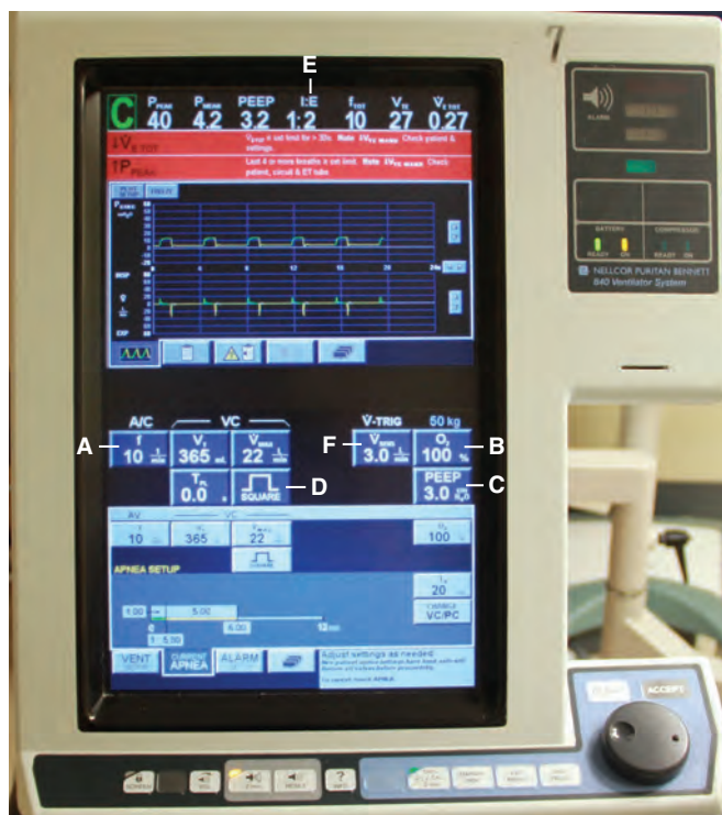
Figure 8.7 The Nellcor Puritan Bennett 840 Ventilator system (Mansfield, MA). Selected features common to all ventilators include the respiratory rate (A), FiO 2 (B), positive end-expiratory pressure (PEEP) (C), waveform (D), inspiratory-to-expiratory ratio (I/E) (E), and trigger (F).
