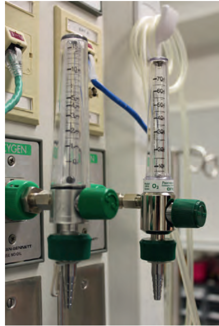
Figure 3.7 A standard flow meter can measure flow up to 15 L/min, but can usually achieve flow rates > 40 L/min when fully opened to "flush"; the maximum possible flow rate is usually marked on the flow meter. Flow meters capable of precisely measuring flow up to 70 L/min are commercially available, which allow the clinician to deliver higher flow rates and thus higher FiO_2 .
