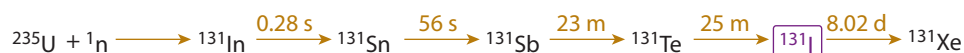
FIGURE A44–1. The decay pathway that describes how ^{131}I is derived from nuclear fuel (whether in a bomb or a reactor) and ultimately decays to stable xenon. s = seconds; m = months; d = days. U = uranium; In = indium; Sn = tin; Sb = antimony; Te = tellurium; Xe = xenon; N = neutron.
