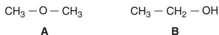
FIGURE 10-8. Two molecules with chemical formula \text{C}_2\text{H}_6\text{O} . (A) Dimethylether. (B) Ethanol (ethyl alcohol).
