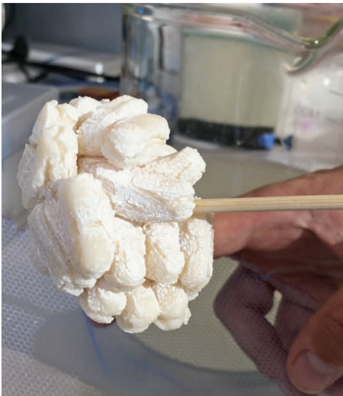
FIGURE 5-2. Pharmacobezoar formation of four different extended-release formulations. A total of 30 tablets were incubated in 1 L of simulated gastric fluid (Ph.Eur., omitting pepsin) for up to 48 hours at 37°C. 286 A , Acetaminophen extended release, 500 mg, 4 hours. B , Acetaminophen combined immediate and extended release, 665 mg, 4 hours. C , Verapamil extended release, 240 mg, 48 hours. D , Quetiapine extended release, 50 mg, 4 hours, and orogastric tube size 30 Fr. (Used with permission from Lotte C. G. Hoegberg as supervisor, mentor and collaborator with Refsgaard F, Petersen SH. In Vitro Investigation of Potential Pharmacobezoar Formation and Their Dissolution of Extended Release Tablets [master's thesis]. Copenhagen: Section of Toxicology, Department of Pharmacy, School of Pharmaceutical Sciences, Faculty of Health Sciences, University of Copenhagen; 2016.)
