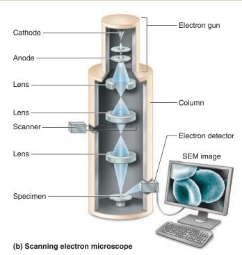
Electron microscopes are large instruments generally housed in a specialized EM facility.
