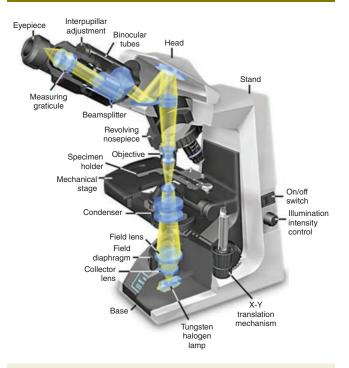
Photograph of a bright-field light microscope showing its mechanical components and the pathway of light from the substage lamp to the eye of the observer. The optical system has three sets of lenses:
